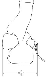
Crystal clear molten glass is poured into a graphite mold to create the sculptural body of the the lamp, which is pierced by a handblown white glass cone and mounted to a bronze armature.
